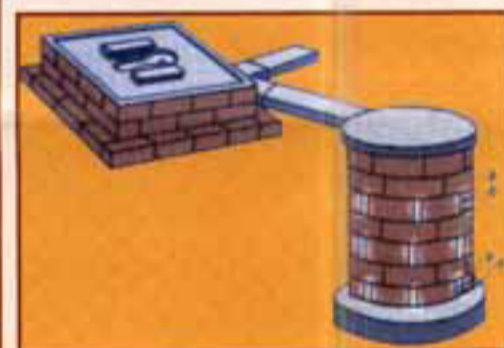
Off Pit Latrine
